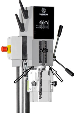
Figure 17 - Grease nipples, drill head
