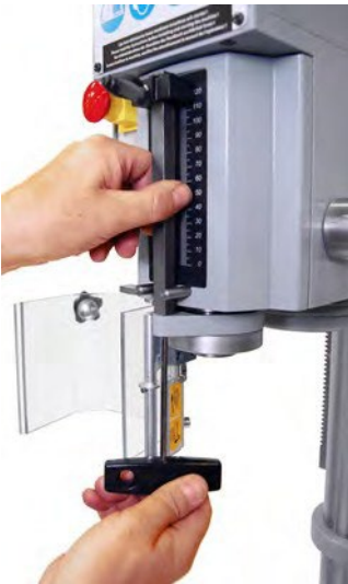
Figure 19 - Removing the depth stop rod
