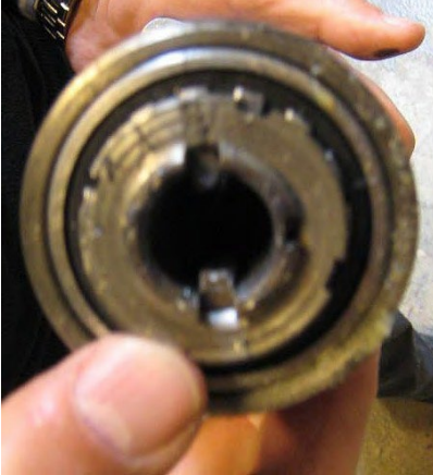
Figure 20 - Nut for adjusting the play of the quill
