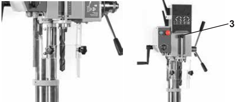
Figure 2a - Chuck guard (for machines within the EU). Figure 2b - Depth gauge (3).
